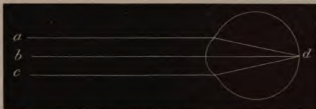
FIG. 427.—Showing concentration of rays of light ( a, b, c ) on the retina ( d ) in normal refraction. (Swanzy.)
